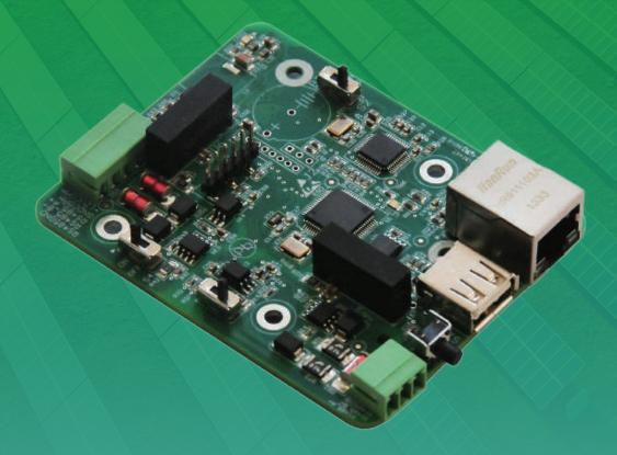
CPS Flex Gateway is a new monitoring and control solution for the CPS 25 to 275kW inverter line.
